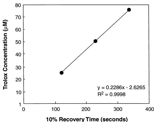
**Fig. 13.4.** Linear relationship between the concentrations of standard Trolox solution ( $\mu\text{M}$ ) and 10% recovery time (sec.).
